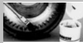
Grease lightly and spread grease evenly. Use a brush.
